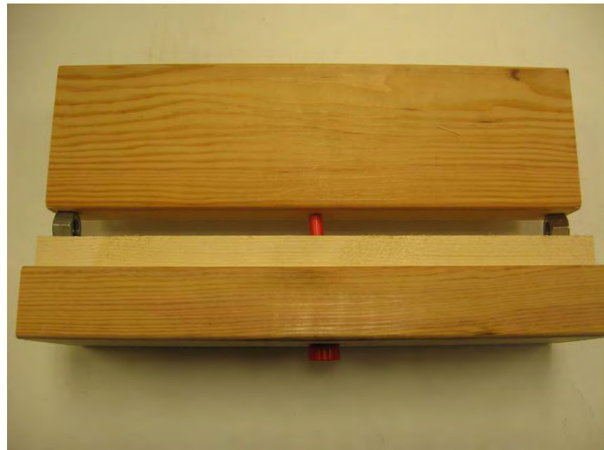
Photo No. 2 Deflector Fastener 3/4" Spacing - Pull-Out Setup
