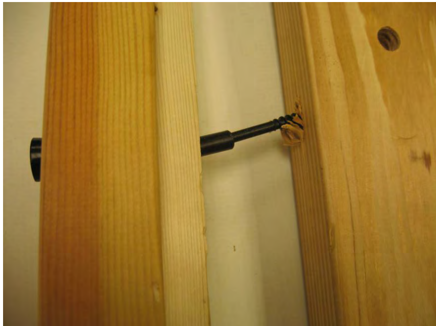
Photo No. 9 Deflector Max Fastener Pull-Out - Failure Detail
