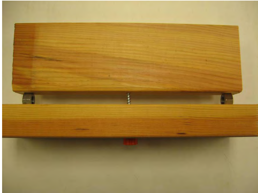
Photo No. 1 Deflector SP Fastener 3/4" Spacing - Pull-Out Setup
