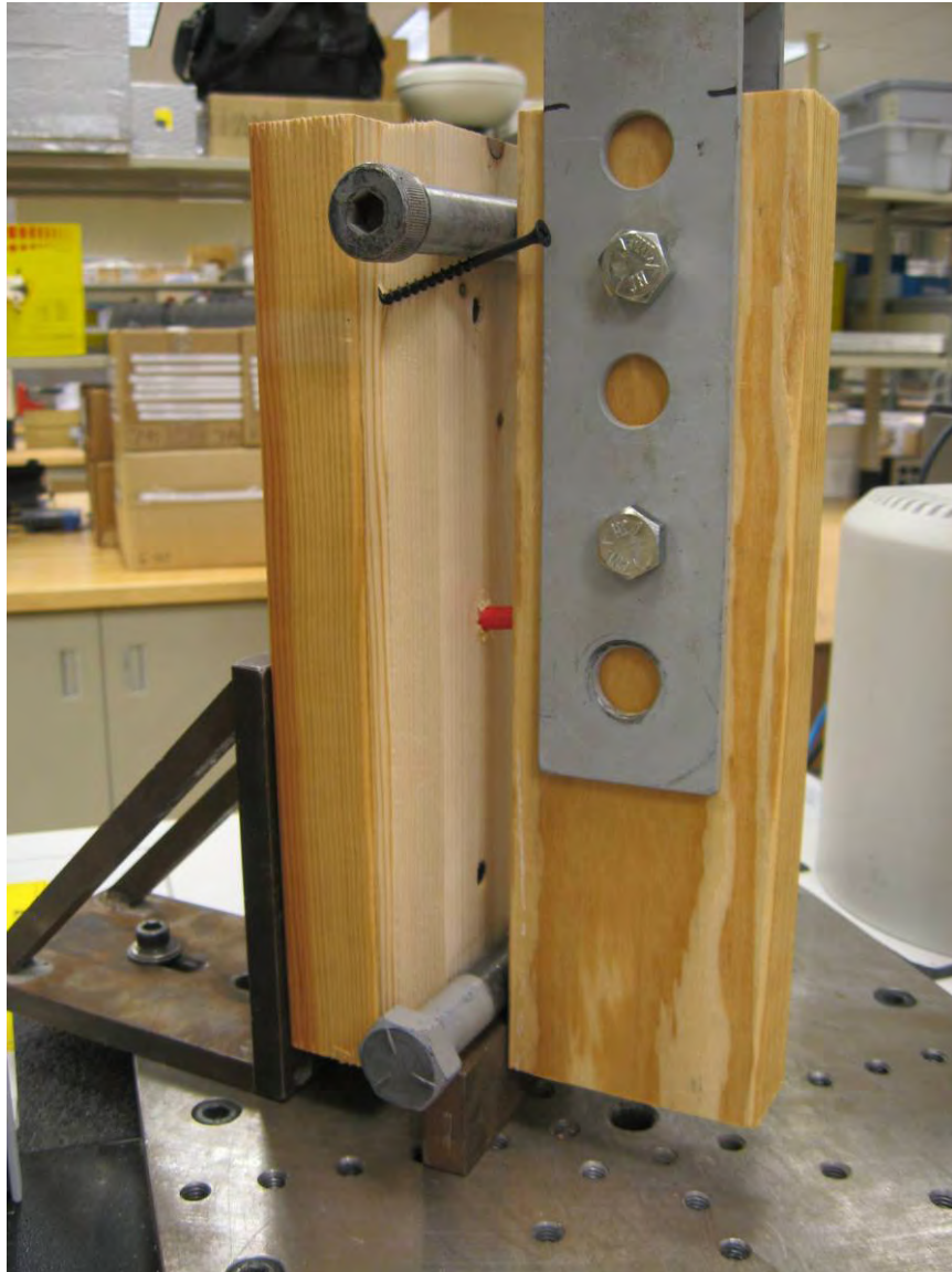
Photo No. 6 Fastener Pull-Out - Setup Detail
