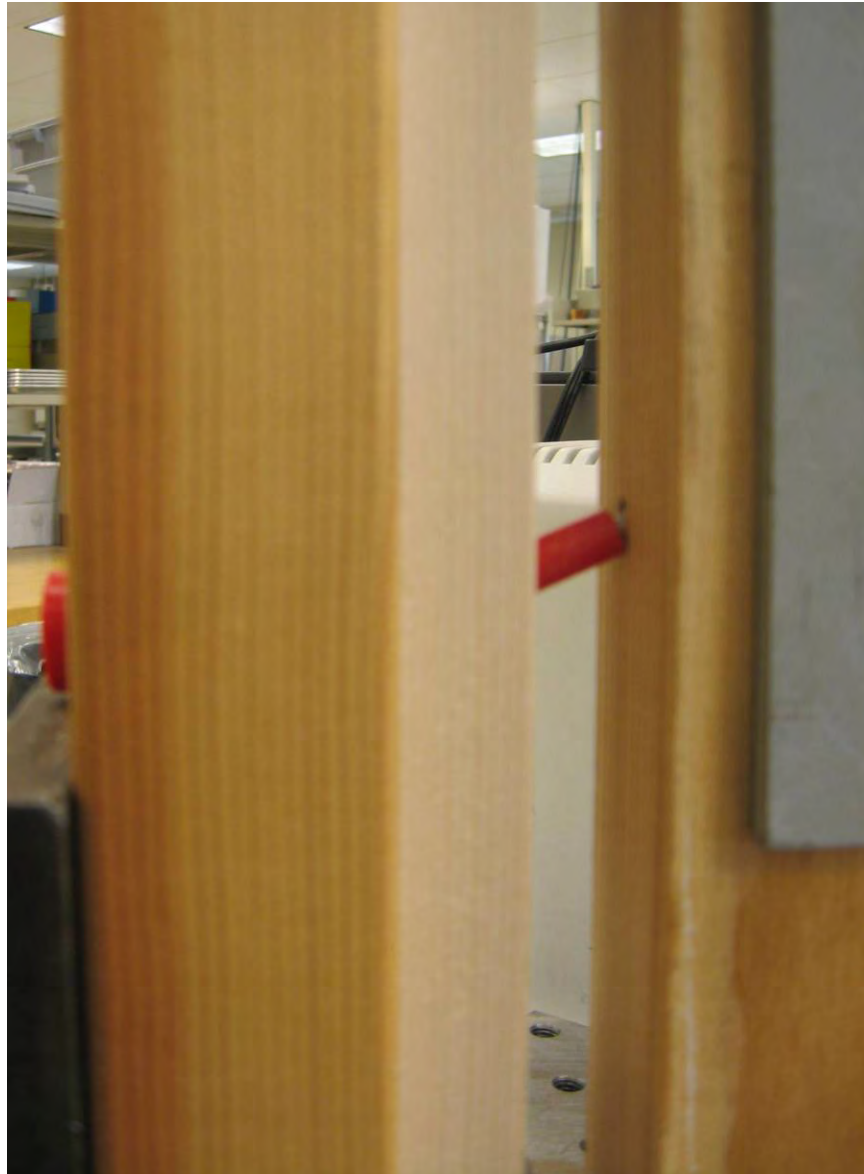
Photo No. 8 Deflector Fastener Pull-Out - Failure Detail
