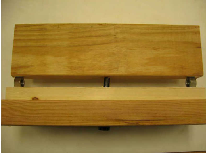
Photo No. 3 Deflector Max Fastener 3/4" Spacing - Pull-Out Setup
