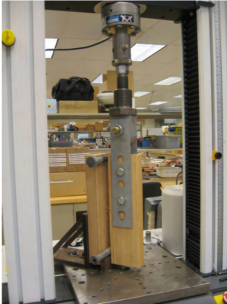
Photo No. 5 Fastener Pull-Out - Setup Detail
