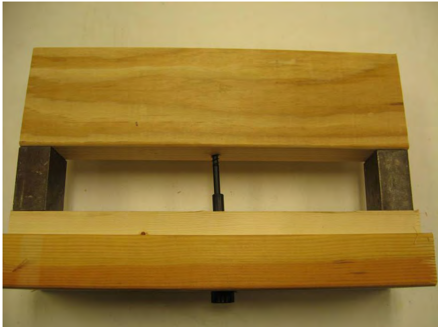
Photo No. 4 Deflector Max Fastener 2" Spacing - Pull-Out Setup
